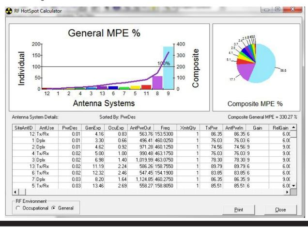
Antennas can be easily activated or de-activated for a particular analysis to predict exposure levels for any particular communications system or individual antenna.
